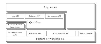
Fig. 4. The QuickStep programming environment
